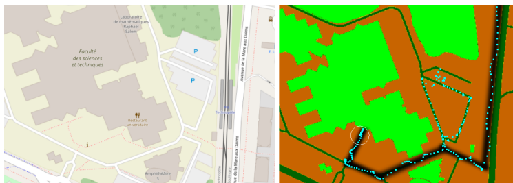
Fig. 3. Left : map from OpenStreetMap. Right: simplified map. The path is a trench (black) that guides user. Building are elevated places, surrounding areas are rough surfaces and other paths are smooth surfaces. The user’s finger is guided by the main path. It is however possible to explore surrounding areas too. The guidance possibilities allow to show the main path in order to help user spatialize it, before letting the user freely explore the area.
